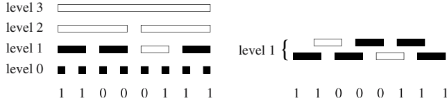
Figure I.6: The building block representation of a H-IFF problem and a one-dimensional, non-circular Ising problem, both with string length 8. All black building blocks are satisfied; all white building blocks are not satisfied.
